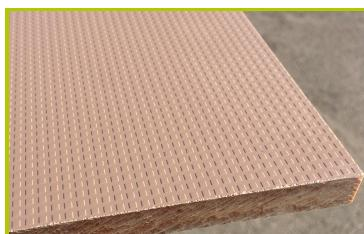
4- **The platforms and the steps** are made from a 12.5mm thick textured and non-slip compact material (HPL).
