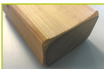
3- **The panels** are made from larch (plank sizes 45 x 68mm). Larch is naturally resistant and long lasting.
