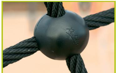
**9- The 16mm diameter ropes** are made of galvanised steel cable covered with polyester. The cables are linked together and held in place by injected polyamide spheres.
