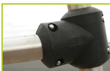
6- **Injection moulded polyamide fixings** connect the posts with the platforms and the various play features. They are non-toxic, flameproof and U.V. resistant. The thickness of the polyamide makes the equipment both strong and vandal resistant.
