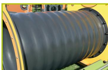
5- **The tunnel** is made of 100% recycled rotomolded polyethylene, 76cm in diameter (RAL 9005).
